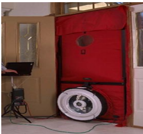
Figure 4 - Set-up equipment of a blower door for the measurement of air tightness (source: Chen et al., 2012)
